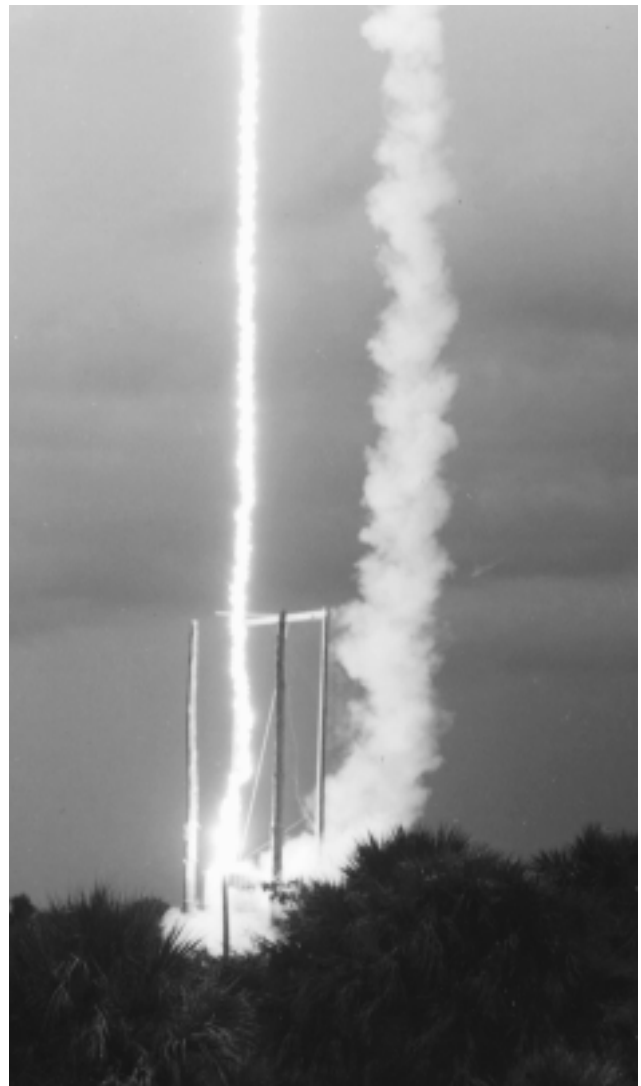
Lightning strikes the RTL launchpad at the Mosquito Lagoon site (bright streak at left) as it follows the vaporized copper wire to the ground after hitting the wire, while the plume of the rocket can be seen to the right. Instruments at the launch pad record the bolt’s characteristics, providing an ideal means to study this phenomenon as it occurs in the environment rather than trying to create the effects in a laboratory.
