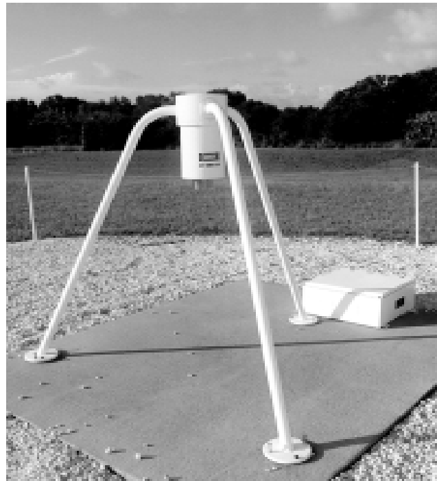
This is one of the 31 electric field mills that comprise the Launch Pad Lightning Warning system. They are called mills because they have a rotating four-bladed shield much like arms of a wind mill. The shield contained in the bottom of the round housing alternately exposes and covers metal sensing plates resulting in an alternating current proportional to the atmospheric electric field.
